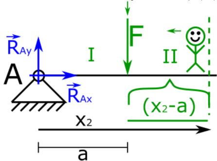
27. We can write final of equation for bending moments in the second section. We need to take first part and add second part.
