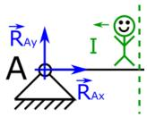
30. We see that at the beginning of the beam there is one force that seems to cut the beam,  $R_{Ay}$  force. Now let's get back to our assumptions, from the beginning, for cutting forces. It can be clearly seen that we are on the left side of the cut, and the sense of  $R_{Ay}$ 's is up, which means that we will take this force with a positive sign.
