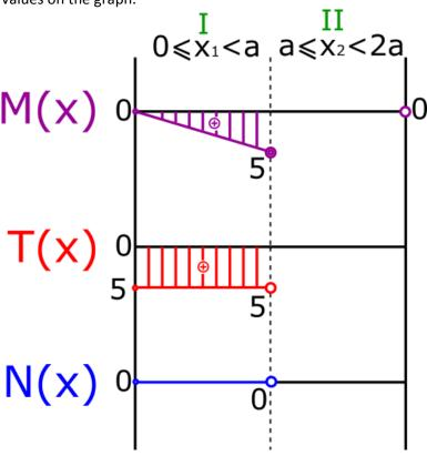
63. Now we consider what kind of function describes the bending moment equation we wrote. It can be clearly seen that this is also a linear equation, what's more it is a descending function. Based on this information, we can connect the points previously marked, mark that we are on the positive side, and finally, we dash this chart.
