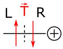
Finally, normal forces remained. For normal forces, the sign depends on whether the forces are directed towards the cut or to the cut. When the forces come out of the beam (the sense is from the cutting point), then we assume that they have positive values. In the opposite case, i.e. when their sense is into the cutting direction (they enter the beam), we assume that these forces have a negative sign.
