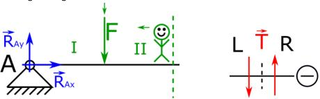
37. We can write final of equation for cutting forces in the second section. We need to take first part and add second part.
