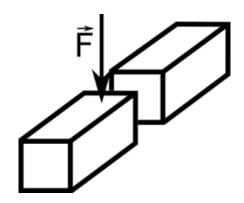
By static beam solution, we mean determining the reactions occurring at the support points and determining the bending moments, cutting forces and normal forces in the beam. These forces are the forces that balance our beam after cutting it.
