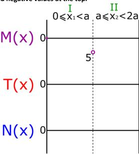
50. Then we consider what kind of function describes the bending moment equation we wrote. It can be clearly seen that this is also a linear equation, what's more it is a growing function. Based on this information, we can connect the points previously marked as shown below.
