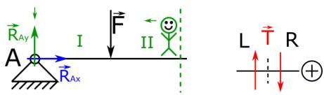
35. We can write first part of equation for cutting forces in the second section. We will write the next part after further considerations.
