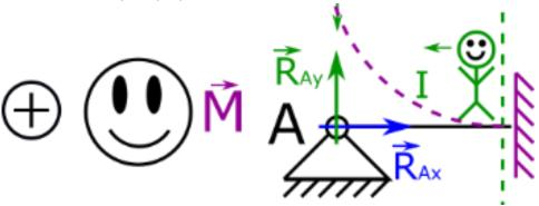
13. According to the notation introduced earlier, if the beam under the influence of force smiles, then we assume that the bending moment from such force is a positive sign. Of course, when cutting, it is clearly seen that we get only half of the smile.
