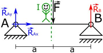
6. After making this cut, we bypass the F force and continue until we come to the  $R_B$  force. Again, something is happening, strength comes to our way, so at this point just before the  $R_B$  force we make the cut again.
