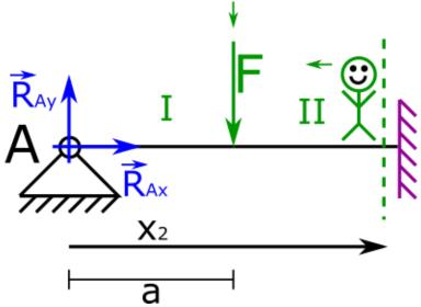
24. At this point, when one end of the beam is fixed, we imagine how the force F tries to bend the beam. You can see clearly in this situation, under the influence of this force, the beam would bend, as shown by the purple dashed line.
