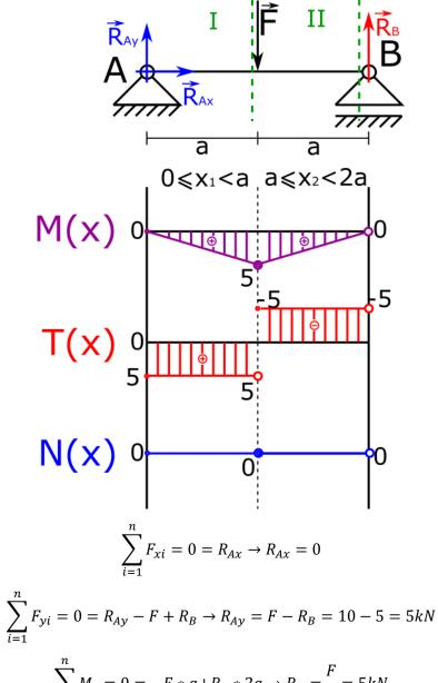
$$\sum_{i=1}^{N} F_{yi} = 0 = R_{Ay} - F + R_B \to R_{Ay} = F - R_B = 10 - 5 = 5kN$$
