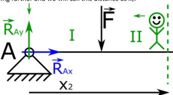
21. We can write first part of equation for bending moments in the second section. We will write the next part after further considerations.
