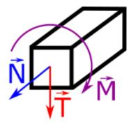
The abovementioned internal forces will be the forces we will count when solving the beams.
