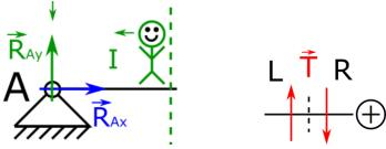
31. After these considerations, we can write the first equation for cutting forces in the first section.
