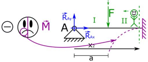
26. We already know what sign the bending moment from F will have, now the arm of this moment should be determined. Because we are standing just before the appearance of the force  $R_B$ , it only means that we are at a distance of difference between  $x_2$  and a from the first section of the beam. The arm of this bending moment will be equal  $(x_2-a)$ .
