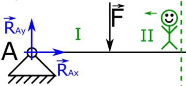
18. We see that at the beginning of the beam there is one force that causes the beam to bend,  $R_{\text{Ay}}$  force.
