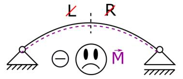
In the case of bending moments, the sign (positive or negative) will depend only on the way the beam is bent, regardless of whether we are on its left or right side.
