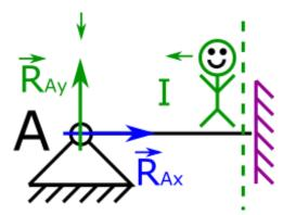
12. At this point, when one end of the beam is fixed, we imagine how the force  $R_{Ay}$  tries to bend the beam. You can see clearly in this situation, under the influence of this force, the beam would bend, as shown by the purple dashed line.
