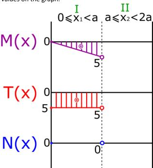
60. Then we consider what kind of function describes the normal forces equation we wrote. It can be clearly seen that this is a constant equation. Based on this information, we can connect the points previously marked as shown below.
