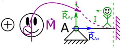
14. We already know what sign the bending moment from  $R_{Ay}$  will have, now the arm of this moment should be determined. Because we are standing just before the appearance of the force F, it only means that we are at a distance of some x from the beginning of the beam. Let's call this distance  $x_1$ , since we're in the first section.
