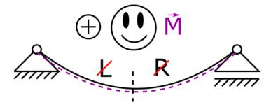
Of course, the beam can also bend upwards, so that the lower fibers (dashed line) are compressed. Then we will assume that such bending moments are negative. It can be said that the beam is sad at the moment, i.e. we have negative values.
