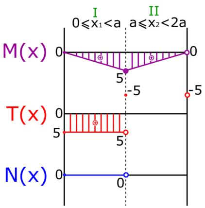
66. Now we consider what kind of function describes the cutting forces equation we wrote. It can be clearly seen that this is also a constant equation. Based on this information, we can connect the points previously marked, mark that we are on the positive side, and finally, we dash this chart.
