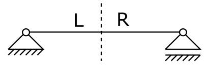
At this point, we will introduce a very important thing, namely the notation according to which we will take positive and negative values of our internal forces: bending moments, cutting forces and normal forces.
