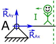
10. We see that at the beginning of the beam there is one force that causes the beam to bend,  $R_{\text{Ay}}$  force.
