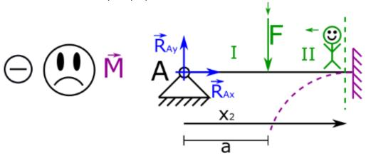
25. According to the notation introduced earlier, if the beam under the influence of force is sad, then we assume that the bending moment from such force is a negative sign. Of course, when cutting, it is clearly seen that we get only half of sad face.
