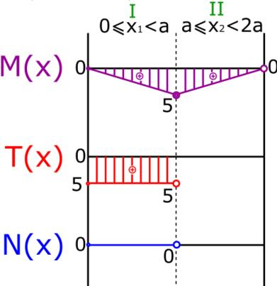
64. We will need the equation of cutting forces for the second section.
