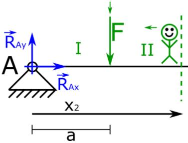
23. Now, to determine how the force bends the beam, we assume that at the place where we stand (where the cut), we catch the beam rigidly.
