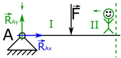
19. Based on the previous section, we can see that this force still bends the beam upwards, hence the moment bending from this force will still be with a positive sign.
