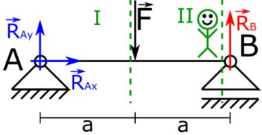
7. In this way, we divided the beam into two sections I and II. The first section within  $0 \le x < a$  second section within  $a \le x < 2a$ .
