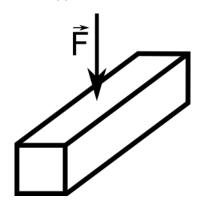
In order to check how the applied load affects the beam deformation, we will have to cut the beam in our thoughts. Such a cut of the beam causes that each of the two parts hangs in the air and in fact would collapse. To maintain system stability, internal forces must be introduced to keep the beam in balance.
