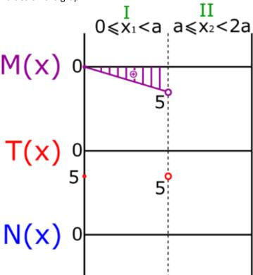
55. Then we consider what kind of function describes the cutting forces equation we wrote. It can be clearly seen that this is a constant equation. Based on this information, we can connect the points previously marked as shown below.
