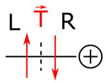
Of course, if on the left side of the cross-section the forces are going down and on the right up, then we have the opposite situation and the cutting forces will be with a negative sign.
