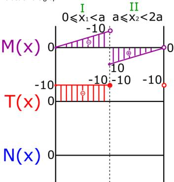
57. Then we consider what kind of function describes the cutting forces equation we wrote. It can be clearly seen that this is a constant equation. Based on this information, we can connect the points previously marked as shown below. We further mark that we are on the negative side. Finally, we dash this chart.
