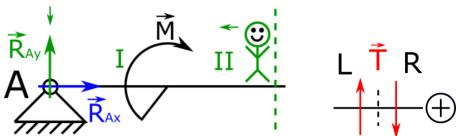
37. We can write equation for cutting forces in the second section. There are no other forces that trying to cut our beam, the only thing left is moment which is not a force this is why we do not include it in the equation of cutting forces.
