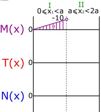
49. Now, unlike the previous examples, we will deal with the equation of bending moments in the second section. And we will consider how the bending moment in the second section changes.
