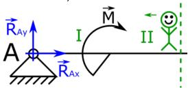
36. We see that at the beginning of the beam there is one force that seems to cut the beam,  $R_{Ay}$  force. Now let's get back to our assumptions, from the beginning, for cutting forces. It can be clearly seen that we are on the left side of the cut, and the sense of  $R_{Ay}$ 's is up, which means that we will take this force with a positive sign. So it is the same, as it was for the first section.
