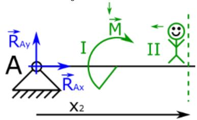
22. Now, to determine how the moment bends the beam, we assume that at the place where we stand (where the cut), we catch the beam rigidly.
