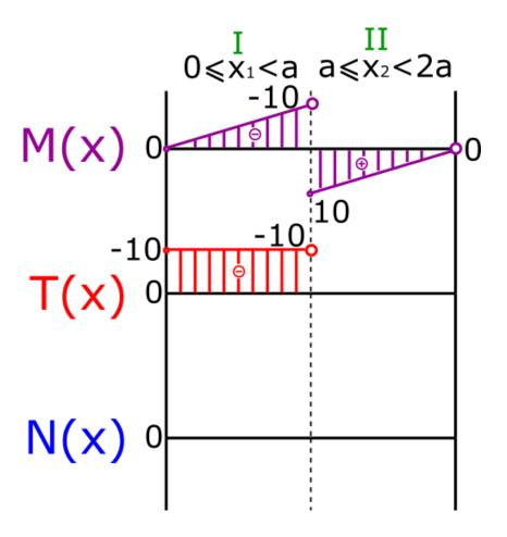
55. Now, unlike the previous examples, we will deal with the equation of cutting forces in the second section. And we will consider how the cutting forces in the second section changes.
