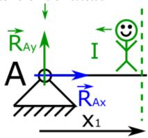
15. After these considerations, we can write the first equation for bending moments in the first section.
