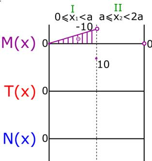
51. Then we consider what kind of function describes the bending moment equation we wrote. It can be clearly seen that this is also a linear equation, what's more it is a descending function. Based on this information, we can connect the points previously marked as shown below. We further mark that we are on the negative side. Finally, we dash this chart. Important information that the lines must be vertical, any other hatching, painting the chart will be incorrect.
