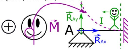
14. We already know what sign the bending moment from R<sub>Ay</sub> will have, now the arm of this moment should be determined. Because we are standing just before the appearance of the force F, it only means that we are at a distance of some x from the beginning of the beam. Let's call this distance x<sub>1</sub>, since we're in the first section.
