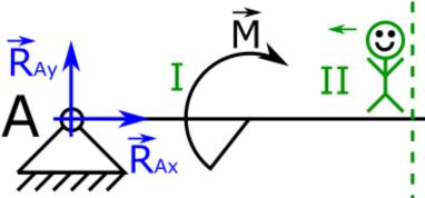
18. We see that at the beginning of the beam there is one force that causes the beam to bend,  $R_{Ay}$  force.
