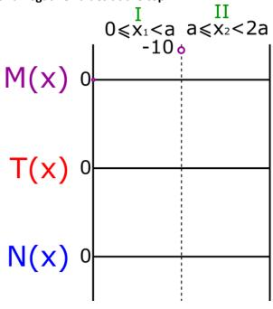
48. Then we consider what kind of function describes the bending moment equation we wrote. It can be clearly seen that this is also a linear equation, what's more it is a descending function. Based on this information, we can connect the points previously marked as shown below. We further mark that we are on the negative side. Finally, we dash this chart. Important information that the lines must be vertical, any other hatching, painting the chart will be incorrect.
