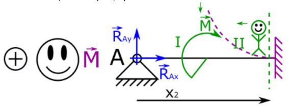
24. We can write final of equation for bending moments in the second section. We need to take first part and add second part. Important information. In the case of a concentrated moment, we do not multiply its value by the arm, but we always place such a moment in the equation of moments.
