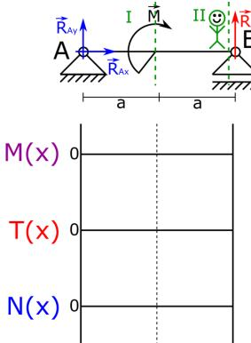
45. In this example, the charts will be drawn step by step so that you can understand their creation. The first graphs will be made for the first section starting from the bending moments graph.
