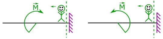
26. We know that a focused moment can be replaced by a pair of parallel forces of the same value and opposite senses that causes rotation around a specific point. As shown in the picture.
