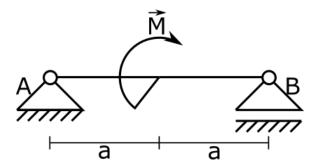
1. The first thing to do when solving beams is to determine the number of supporting unknowns, as was the case with trusses. It is clear that in this case we have three unknown supports. In addition, you must specify how we will adopt the coordinate system in accordance with which we will determine the values of supporting unknowns and in which direction the moments will have positive values. In this case, anticlockwise turning moments will be positive.
