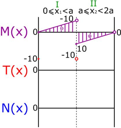
54. Then we consider what kind of function describes the cutting forces equation we wrote. It can be clearly seen that this is a constant equation. Based on this information, we can connect the points previously marked as shown below. We further mark that we are on the negative side. Finally, we dash this chart.
