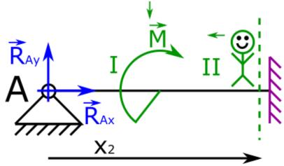
23. At this point, when one end of the beam is fixed, we imagine how the moment M tries to bend the beam. You can see clearly in this situation, under the influence of this moment, the beam would bend, as shown by the purple dashed line.
