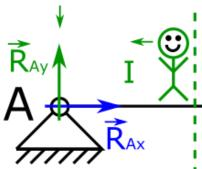
11. Now, to determine how the force bends the beam, we assume that at the place where we stand (where the cut), we catch the beam rigidly.
