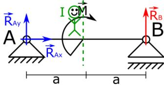
6. After making this cut, we bypass the M moment and continue until we come to the  $R_B$  force. Again, something is happening, force comes to our way, so at this point just before the  $R_B$  force we make the cut again.
