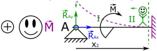
20. We can write first part of equation for bending moments in the second section. We will write the next part after further considerations.
