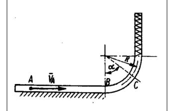
m=0.2kg  $V_A=10m/s$   $t_{BD}=1s$  R=0.5m  $\mu=0.1$   $\alpha=60^\circ$   $k=1.2\,N/cm$ Additionally find, h
