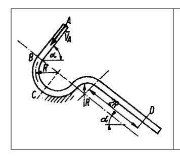
$m = 0.8 \ kg$   $V_A = 3m/s$   $t_{AB} = 0.2s$  R = 0.4m  $\mu = 0.15$   $\alpha = 45^{\circ}$ Additionally find,  $V_D$
