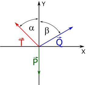
Now we can write equation of equilibrium for planar convergent system. It is known that for planar convergent system we can write two equilibrium equations. In this system there are two unknowns so it is possible to solve it.
