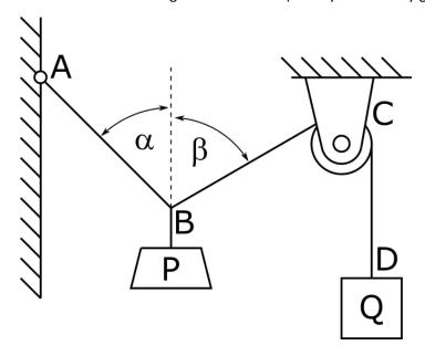
2. Next we can introduce forces that are acting in the system. It is clearly seen that between points A and B must be some tension (force). What is more this force T must acting exactly along direction of AB, what is shown in the picture.
