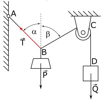
The sense of force T was determined based on the intuition and drawing itself. One can noticed that all forces except of force T are acting downwards, so force T must acting upwards, along its direction. What is more it one can found that force Q are acting not only at point D but actually, at the whole distance from point B through point C up to point D. This is why we can reduce this system to the simple convergent system at point B. As it is shown below.
