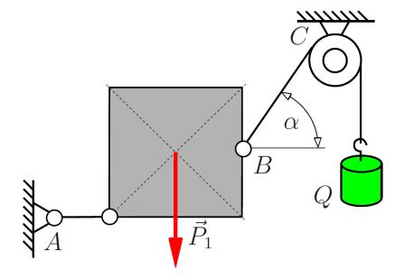
3. The stiff rod was connected to the ground at point A by the joint and to the rope at point B. Additionally at point B mass Q was attached. Calculate the value of the force P1 and the forces in the other rods and ropes SAB, SBC, SCD if the system is in equilibrium as in the drawing. Data: Q = 300 [kg],  $\alpha$  = 30°,  $\beta$  = 45° Unknown: P<sub>1</sub>.
