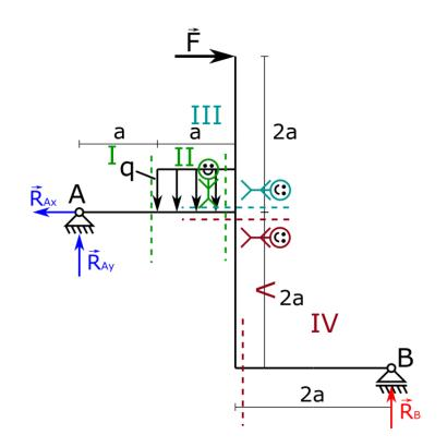
6. The last thing to do before starting to write equations in each of the intervals is to **mark** where on each part of the frame we will take its bottom. In this case it has been marked with an orange dashed line. This step is very important because it allows us to tell if a given part of the frame is smiling or has a sad face as it was in the case of beams. This information is needed to be able to correctly write the bending moment equation.
