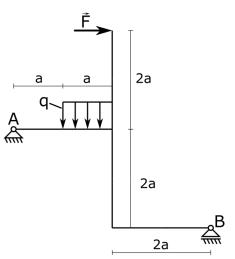
In this case, we have frame with one stable support and one movable support but we also have a place where the frame parts cross. As for beams, we must first identify support unknowns. In addition, you must specify how we will adopt the coordinate system in accordance with which we will determine the values of supporting unknowns and in which direction the moments will have positive values. In this case, clockwise turning moments will be positive.
