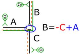
26. Finally, in the resulting equation, we insert the bending moments obtained earlier for each part of the frame in the place of the intersection and check that the left side is equal to the right. If the sides of the equation do not match, it means that in one of the earlier steps we made a mistake.
