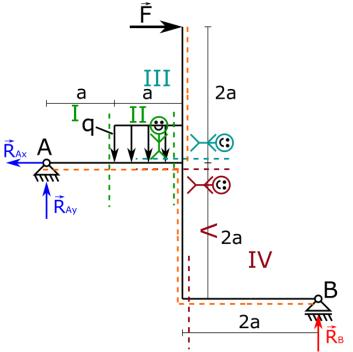
7. In this way, we divided the beam into five sections. The first section within  $0 \le x < a$ , second section within  $a \le x < 2a$ , third section within  $0 \le x < 2a$ , fourth section within  $0 \le x < 2a$ , fifth section within  $0 \le x < 2a$ .
