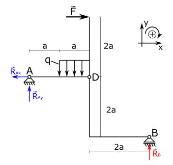
$$\sum_{i=1}^{n} M_{D} = -R_{B} * 2a + R_{Ay} * 2a + F * 2a - qa * 0,5a = -\frac{19}{4}qa^{2} - \frac{11}{4}qa^{2} + 8qa^{2} - \frac{2}{4}qa^{2} = 0$$
