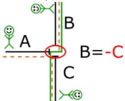
25. Then go to part A and perform a similar operation. We want to go to beam B so that we are on the upper part (green line). It is clear that we do not cut the beam A or beam B in any way (marked in blue). Therefore, the sign at the moment bending from beam A will remain as it was.
