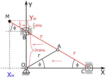
8. Finally, we can write the equation to the YM coordinate as follows.
