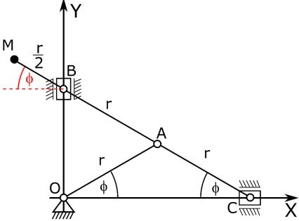
4. Once we have a well-described geometry of the mechanism, we can move on to determining the equations of motion. To do this, you need to define its  $X_M$  and  $Y_M$  coordinates, respectively, based on the given position of the M point, as shown in the figure.
