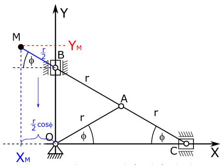
6. The negative sign in the equation results from the fact that the point M is on the negative side of the X axis coordinates, which is clearly visible in the next figure.
