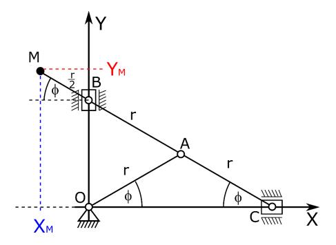
5. Let's start with determining the coordinate on the X axis. In this case, to do this, project the MB segment onto the OX axis. We will then obtain the equation of the following form,
