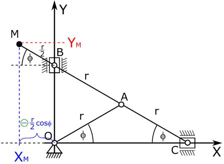
7. Once we have a specific value of the coordinate on the X axis, we can go to the Y axis. Similarly to the previous case, we also project the geometry to the Y axis as shown in the figure.
