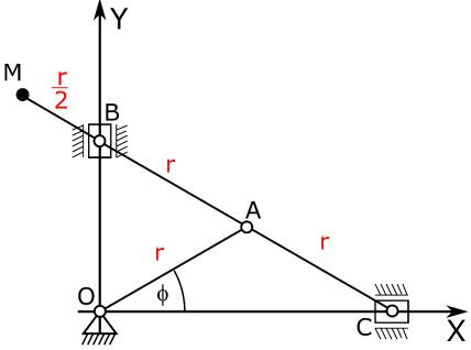
2. Then it is clearly seen that an isosceles triangle was formed, hence it can be seen that we will also have an angle at point C  $\phi$ .
