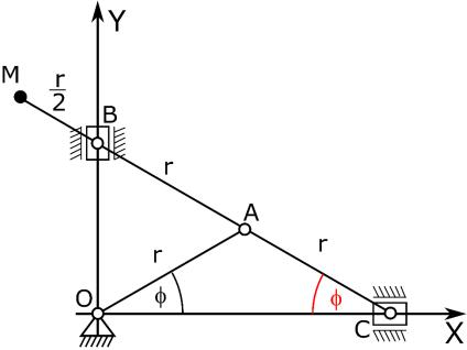
3. Analyzing the drawing further, it can be seen that the same angle will be at point B as shown.
