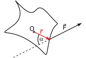
5. The vector product of vectors r and F will be called as a moment M of a vector F related to point O. The resultant vector of mentioned vector product will be perpendicular to the plane on which vector r and F are placed, and the sense of this vector will depends if we are rotating clockwise or anticlockwise.
