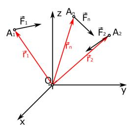
3. Next at point O we will introduce pairs of vectors (zero pairs) in, a way that do not have influence on the system.
