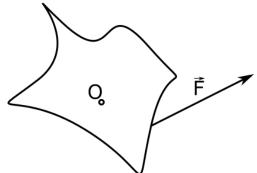
2. One can see that the direction of this force is not going through the O point which is interesting for us. It can be said that force F is acting on point O not directly but indirectly.
