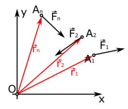
In case of planar system of force we can reduce such a system to one resultant force S
