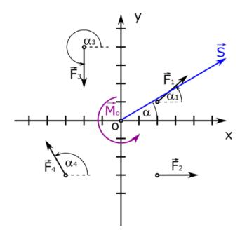
4. Next we can find equation of the straight along which the resultant force works, and the distance of the direction of the resultant force from the center of reduction.
