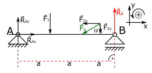
The only thing left is to determine sign for the moment from this force. Let's do the same as we did for first force, so we will use our imaginary compass. As you can see force  $R_B$  is trying to rotate around point A anticlockwise. Moment from this force will be positive, because we assume at the beginning that positive sign of moment will be for anticlockwise rotation. Now we can include moment from this force in our equation.
