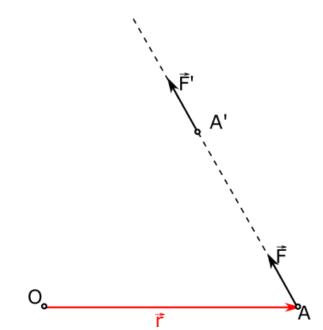
9. If we want to calculate moment for this new position of vector of force we need to introduce new vector r' in order to have "arm" vector.
