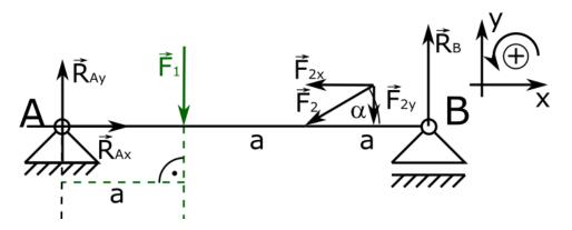
After finding distance you need to determine if the moment from this force will be with positive or negative sign. The best way is to imagine yourself that you have compass, and one end of a compass you are attaching to the point around which force is trying to rotate, and second end you are trying to rotate according to the sense of the force.
