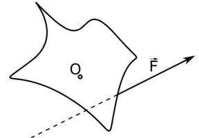
3. Due to the fact that this force is acting indirectly we need to know how we can find influence of the force on point O. Let introduce vector r, which is connecting point O and the force which is acting on it. We can call vector r as an "arm".
