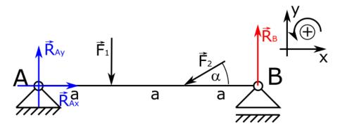
2. We have three unknowns and we know that this system is in equilibrium state. Additionally this is planar system, so we can write three equations of equilibrium. Projection of forces over axis X, projection of forces over axis Y and sum of moments relative to point. We can pick any point we want, but later I will write which point we will choose and why.
