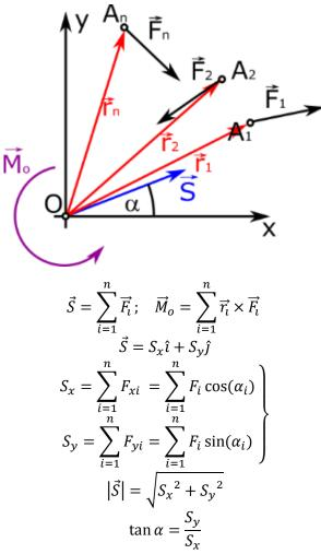
$y = \frac{S_y}{S_x} * x - \frac{M_0}{S_x}$  the equation of the straight along which the resultant force works  $r = \frac{M_0}{S}$  distance of the direction of the resultant force from the center of reduction
