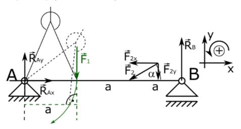
As you can see force  $F_1$  is trying to rotate around point A clockwise. Moment from this force will be negative, because we assume at the beginning that positive sign of moment will be for anticlockwise rotation. Now we can include moment from this force in our equation.
