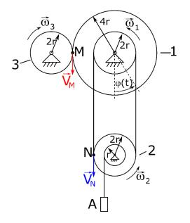
Finally, we turn to point A. It is clearly visible that the linear shift of point A will be equal to the length of the rope unwound from the arc s.
