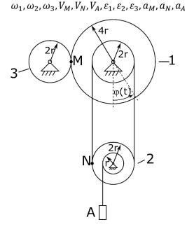
First we determine the angular velocity and angular acceleration for wheel 1. And then the linear velocity for point M. It can be seen that this point belongs to wheels 1 and 3, therefore the linear velocities will be the same.
