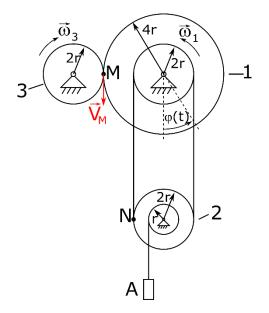
Then we can look at point N. The point is connected to wheel 1 by a transmission belt. Therefore the linear velocity on the circumference of the smaller wheel 1 will be the same as the velocity of point N.
