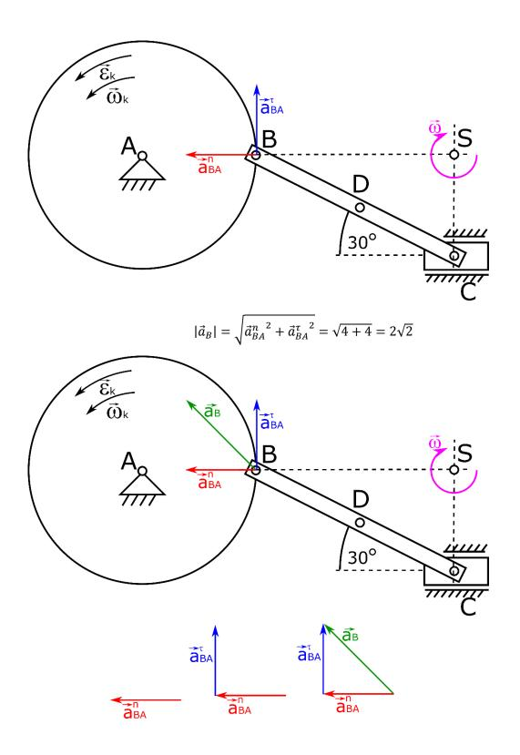
Then we calculate the acceleration for the remaining points. First choose from which point C or D we start. You can see that, as in the case of velocity, also here point C can only move horizontally, so its acceleration will be in this direction.
