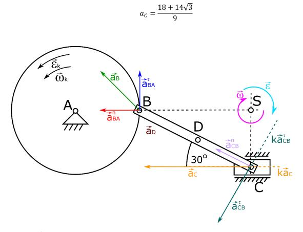
Having information about the angular velocity and the angular acceleration, we can calculate the acceleration of point D. We do not know the direction of this acceleration, but we will know the values and directions of the components of this acceleration.
