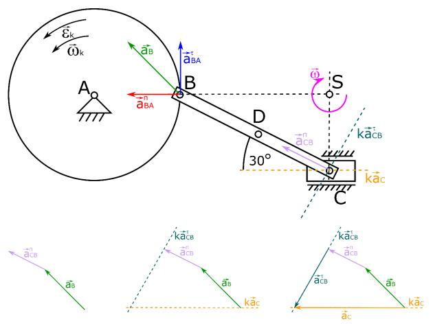
In the next step, we project the accelerations on the X and Y axes and in this way we are able to determine the acceleration of point C and the tangential acceleration of point C with respect to B. By determining the tangential acceleration, we can find the value of the angular acceleration.
