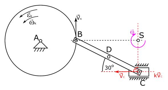
After determining the velocity of point B and finding the angular velocity, we can determine the velocity of point D. We run a straight line from point S to point D and the velocity vector of this point will lie on the perpendicular direction.
