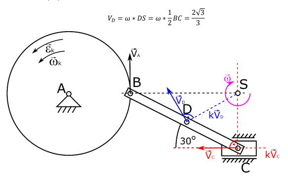
Next, we can move on to determining the accelerations. We'll start with point B. It's on a circle whose center is stationary, so we'll calculate the acceleration of point B about the center of the circle.
