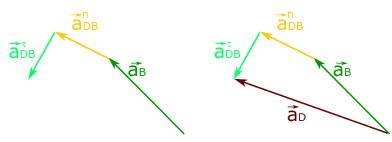
In the next step, we project the accelerations on the X and Y axes and in this way we are able to determine the acceleration of point D. It is true that we first determine the values of its components on the X and Y axes, but determining the final value of acceleration D is then a formality.
