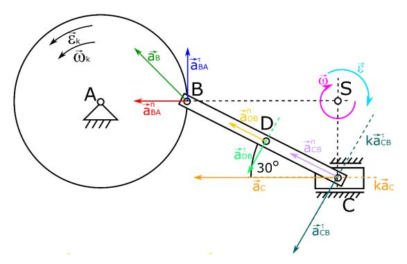
After plotting these accelerations on the drawing, we can create a chain of accelerations, just like in the case of point C.
