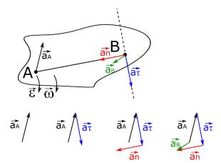
In the figure below, you can see the similarity of plane motion to circular motion.
