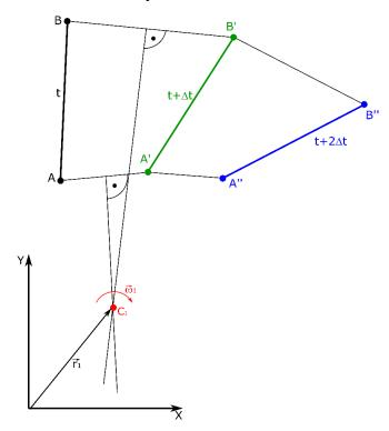
If we now connect once again the corresponding points with straight lines, and then draw the lines perpendicular, we will notice that the lines will intersect at one point. Let's call this point C<sub>2</sub>.
