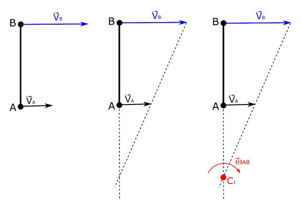
Velocities directions parallel to each other. The velocities have the different sense, might have same or different value. We draw two lines connecting the beginnings of velocity vectors and their ends.
