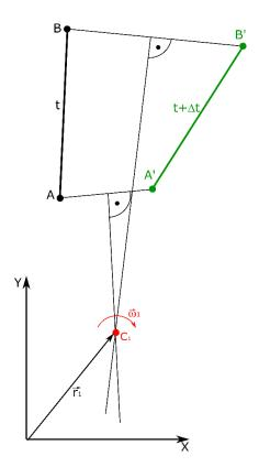
The determined point  $C_1$  will be called the instantaneous center of rotation (or temporary rotation point (TRP)).
