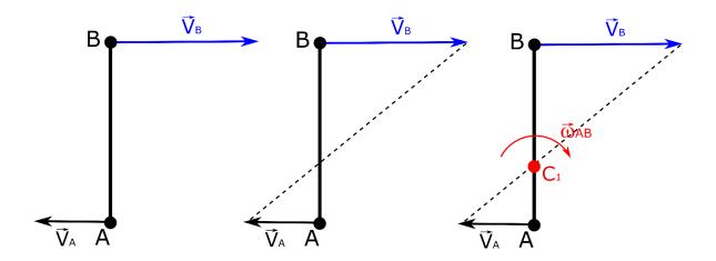
Velocities directions parallel to each other. The velocities have the same sense and same value. We draw two lines connecting the beginnings of velocity vectors and their ends. As you can see, the drawn lines will not cross. This means that the instantaneous center of rotation is infinity and the angular velocity is zero. The body only makes a translational movement.
