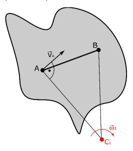
Then, in the direction perpendicular to the previously drawn section, we find the velocity of interest. The sense of velocity will be in the direction of rotation of the angular velocity.
