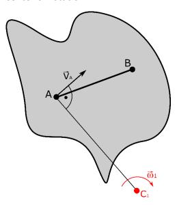
Knowing the location of this point, we can easily determine the velocities for other points of interest to us. For this purpose, a straight line should be drawn from the temporary rotation point to the point of interest.
