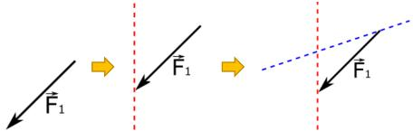
11. Based on obtained triangle we can establish values and senses of reactions. Because all forces must creating closed triangle of forces. It will look as follows.
