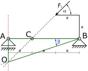
17. In this way we obtained a new triangle CAO, where sides AC and AO must be equal to each other. It means that distance AO is equal to a.
