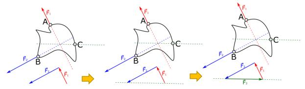
Due to the fact that our rigid body is in balance the triangle of forces must be closed. And in this way we know value and the sense of each force.
