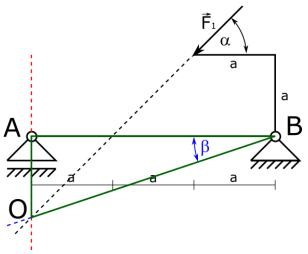
16. We know that the distance AB is equal to 3a, it is hard to say something about distance OB, but we have some information about distance OA. We should remember that angle  $\alpha$  is 45° it means that direction of force  $F_1$  is going through the distance AB exactly between a and 2a, at point C.
