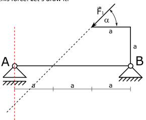
8. We just found the point where directions of two forces are crossing. Due to the fact that this body is in a balance it means that the direction of third force (reaction at point B), must going through this point as well. Let's draw it.
