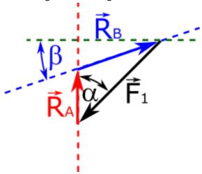
20. Now we now three angles in our triangles and we can calculate values of reactions using theorem of sines.
