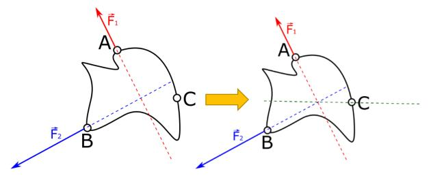
And next based one the triangle of forces we can determine value. In order to construct triangle of forces we need to draw two forces that we know, and then add the direction of third force, or if we know only one force we are adding direction of other two forces, in a way, that these directions are going through the beginning and end of known force.
