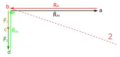
13. Next we are still rotation, and reaching rod 1. There is the same situation as with rod 2, so we do not know value of force but we know direction. We are drawing direction of this force, as it is shown in the figure. We can see that between rod 2 and rod 1 is area "f", and between rod 1 and force  $R_B$  is area "a".
