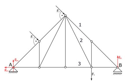
$$\sum_{i=1}^{n} F_{xi} = 0 = -R_{Ax} + F_1 \cos 45^\circ + F_2 \cos 45^\circ \to R_{Ax} = 21,15kN$$
