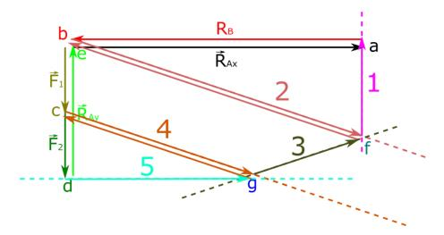
26. Now, we know sense of force in rod 5 next to this point, and we can draw it, in a way it was done above for other rods. Base on the figure we can say that rod 5 is compressed.
