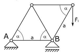
1. In order to start solving truss we will mark and count number of unknown reactions. In this example, we have 3 unknown reactions.
