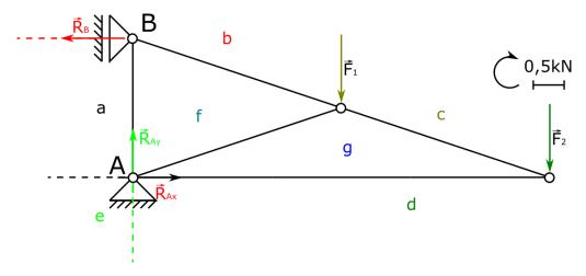
6. First of all, we will "walk around" our truss from the outside. We need to start at some point. Let's start at point A (area "a"). We can see that at this point we have force R<sub>Ax</sub>. We need to draw this force according to the established scale. At the end of this force we mark that it is touching area "a".
