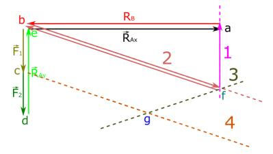
21. We can see that, there are no other forces at this point. It means that forces in rod 2 and  $F_1$ , and directions of these two other forces must crate closed chain of forces. This is why we know what are the senses of each of these forces, and we can draw them in the figure.
