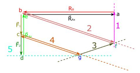
25. We can see that, there are no other forces at this point. It means that forces in rod 4 and F<sub>2</sub>, and directions of third force must crate closed chain of forces. This is why we know what is the sense of last force, and we can draw it in the figure.
