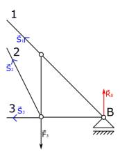
7. Now when we have two parts with introduced unknown forces we need to choose one: left or right. I suggest to choose part where is the smallest amount of forces. In order to make calculations easier. In this case we will take left part of truss (in blue circle).
