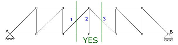
3. Next rule is that three rods through which you are cutting must not starting in one joint. This is why cut done in first example is incorrect.
