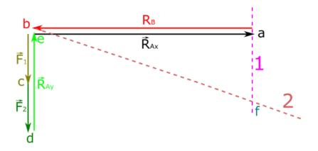
14. We can see that, there are no other forces at point B. It means that force R<sub>B</sub>, and directions of these two other forces must crate closed chain of forces. This is why we know what are the senses of each of these forces, and we can draw them in the figure.
