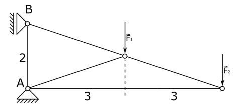
1. In order to start solving truss we will mark and count number of unknown reactions. In this example, we have 3 unknown reactions.
