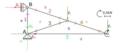
24. At this point we will start with force which is in rod 4. Because next to this point sense of force in rod 4 will be opposite to the previously drawn, we need to draw this force once again with proper sense, as it was shown in figure. Next, we have fore F<sub>2</sub> and it is already drawn. After that we are reaching rod 5, where we know only direction, which we are drawing, as it was shown in figure.
