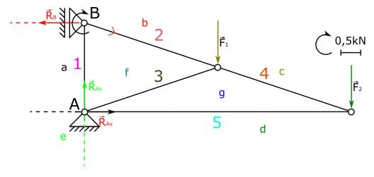
16. Due to the fact that rods are symmetrically loaded we need to draw second arrow next to the second end of rod 2 however, with opposite sense to the first one, as it was done in figure. Now, based on this arrows (inner forces), we can say that this rod is stretched. Now we need to do the same thig for force in rod 1. As you can see this rod is compressed.
