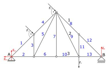
3. Third we will mark, and count number of joints. This truss has 8 joints.
