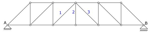
2. This cut should be done through 3 rods. But it must be done in a specific way. The cut that you will done must divide truss to two parts. As you can see below there are two examples. First is done badly, because as you can see cut is done through 3 rods, however, it does not dividing truss to two parts. This is why you cannot cut like that.
