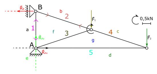
18. At this point we will start with force which is in rod 2. Because next to this point sense of force in rod 2 will be opposite to the previously drawn, we need to draw this force once again with proper sense, as it was shown in figure. Next, we have fore F<sub>1</sub> and it is already drawn. After that we are reaching rod 4, where we know only direction, which we are drawing, as it was shown in figure.
