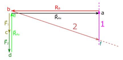
15. Now, we know senses of forces in rods 1 and 2 next to the point B, and we can draw them. In order to make it simpler I will start from force in rod 2. We need to take sense of force 2 from our chain of forces and place it next to the point B, as it was done in figure (arrow on rod 2)
