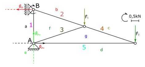
12. At point B we have force R<sub>B</sub> which is already drawn. Now, we are rotating clockwise and we are reaching rod 2. We do not know the value of force in this rod but we know the direction of this force. This is why we are drawing it, as it is shown in the figure. We can see that between force R<sub>B</sub> and rod 2 is area "b".
