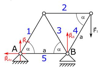
3. Third we will mark, and count number of joints. This truss has 4 joints.
