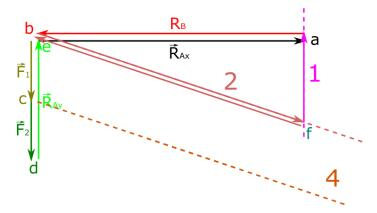
19. Next we are still rotation, and reaching rod 3. There is the same situation as with rod 4, so we do not know value of force but we know direction. We are drawing direction of this force, as it is shown in the figure.
