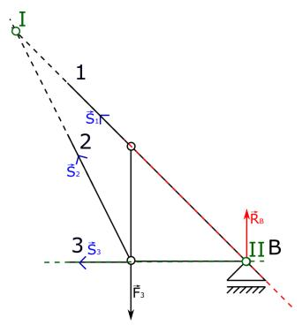
11. Third pole. Directions of S₁ and S₃ are extended, and at the point where they are crossing we are introducing third pole (green point III).
