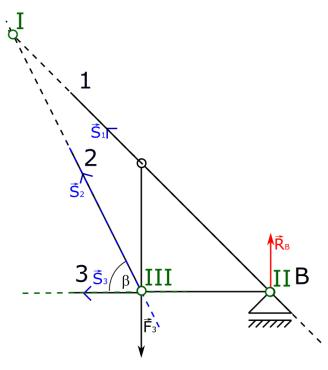
12. After establishing three poles, we need to check if these points are not lying in one line. If this condition is met, we can write equations of equilibrium for our system.
