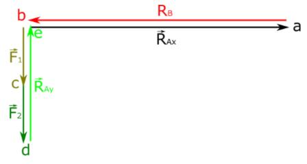
At this point we can see that we have made a whole circle around our truss, because if we will keep rotating we will start from the beginning (force  $R_{Ax}$ ).
