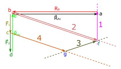
22. Now, we know senses of forces in rods 3 and 4 next to this point, and we can draw them. In a way it was done above for rods 1 and 2. Base on the figure we can say that rod 4 is stretched and rod 3 is compressed.
