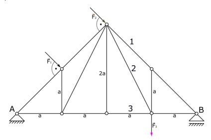
1. For each truss beginning is the same (check if we can solve it in static way). In order to start solving truss we will mark and count number of unknown reactions. In this example, we have 3 unknown reactions.
