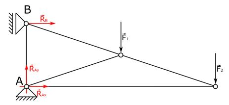
Of course we also need to calculate number of rods and joints. We can see that there are 5 rods and 4 joints, so this truss might be solved with static methods. Because
