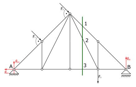
6. Let's divide truss to two separate parts. At this point we need to introduce forces to the rods through which cutting was done, in order to keep system in a balance. These introduced forces are our unknowns. WE ARE NOT INTRODUCING FORCES TO OTHER RODS.
