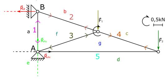
23. Next point is a point where force F<sub>2</sub> is applied (you can see rotation marker). This will be our final point, because based on this point we can establish last unknown force it is force in rod 5.
