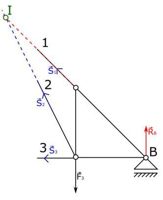
10. Second pole. Directions of  $S_1$  and  $S_3$  are extended, and at the point where they are crossing we are introducing second pole (green point II).
