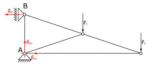
3. Next, we need to divide our truss to areas, as it was shown in the figure. Each area is between directions of forces. The best way is to start from the outside, and then move around our truss. After marking area on the outside we can mark inner areas. For example: area "a" is between directions of R<sub>Ax</sub>, R<sub>B</sub>, and rod between points A and B. In order to make it easier to understand I marked each area with different color.
