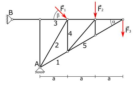
4. Find reactions in supports and forces in marked rods. Use joints and Ritter's methods. Data:  $F_1$ =4kN,  $F_2$ =5kN,  $F_3$ =2kN, a=1m, h=3m
