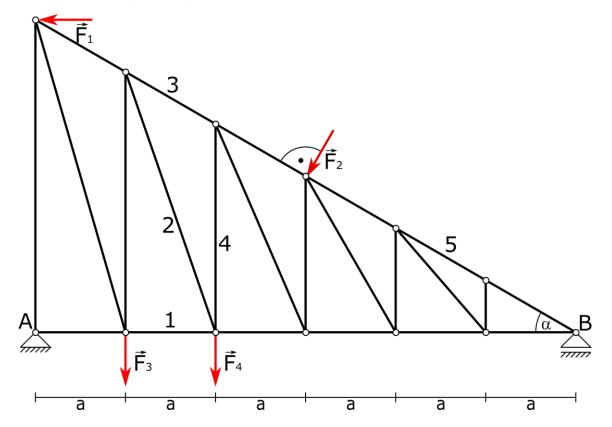
3. Find reactions in supports and forces in marked rods. Use joints and Ritter's methods. Data:  $F_1$ =4kN,  $F_2$ =2kN,  $F_3$ =5kN, a=1m,  $\alpha$ =30°,  $\beta$ =45°.
