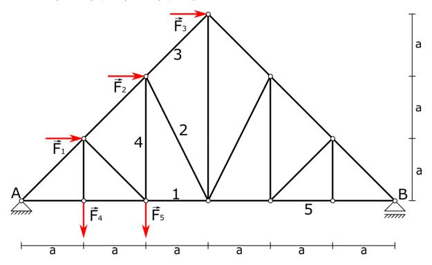
2. Find reactions in supports and forces in marked rods. Use joints and Ritter's methods. Data:  $F_1=5kN$ ,  $F_2=2kN$ ,  $F_3=3kN$ ,  $F_4=4kN$ , a=1m,  $\alpha=30^\circ$ .
